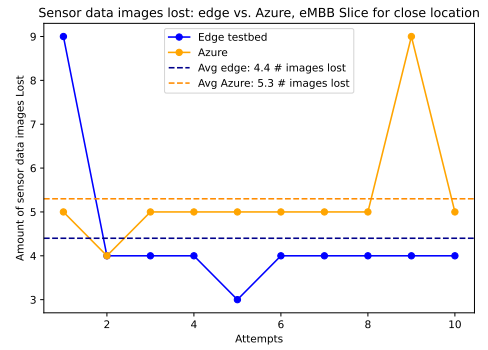
Fig. 6: Amount of file losses for close location, eMBB slice edge vs. Azure.
