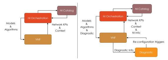
Fig. 3: Two strategies for control loops between NI instances and NI Orchestration layer.
