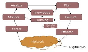
Fig. 4: Extended MAPE-K abstractions for NI algorithms.
